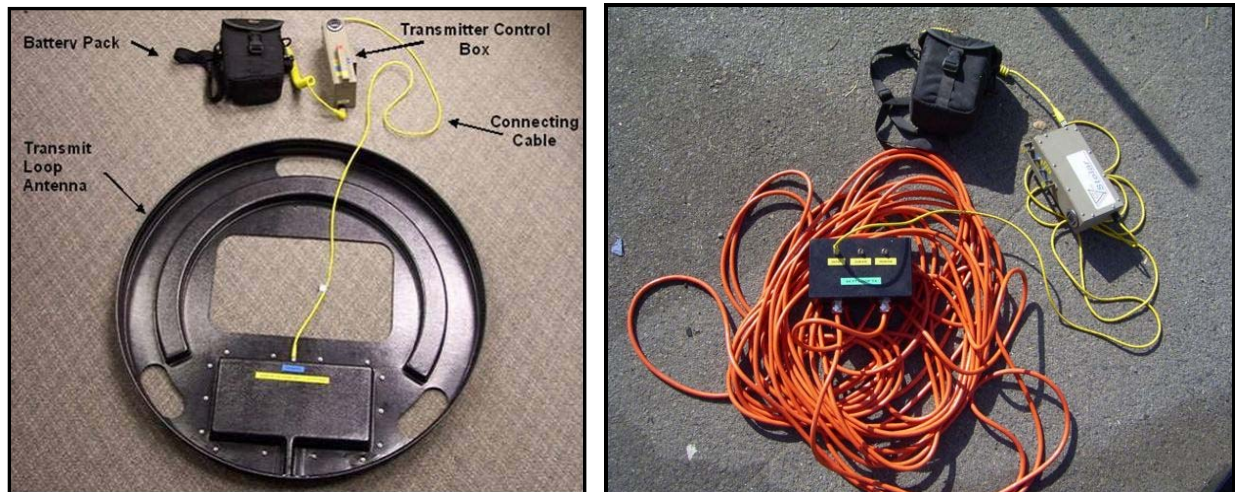
Figure 4. DeltaEM Gradiometer system transmitter components; 30-in.-diameter loop (left), and 31-ft-diameter loop coiled up (right).
